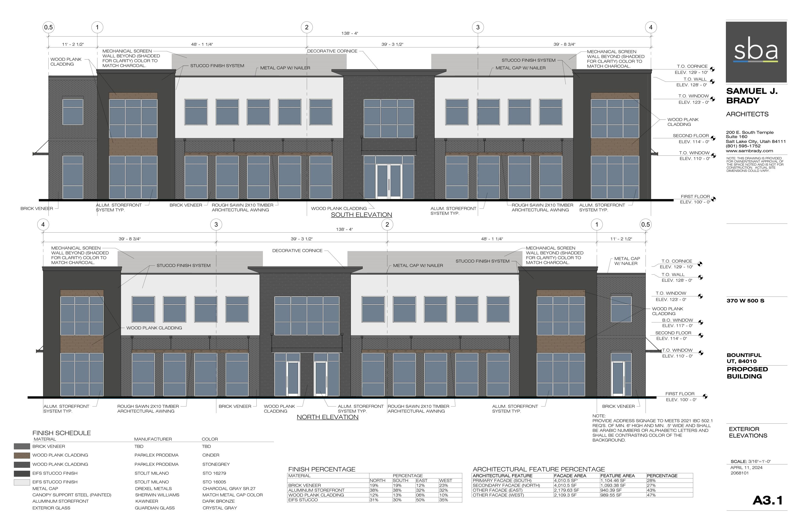
NOTE: PROVIDE ADDRESS SIGNAGE TO MEETS 2021 IBC 502.1 REQ'S. OF MIN. 6" HIGH AND MIN. .5" WIDE AND SHALL BE ARABIC NUMBERS OR ALPHABETIC LETTERS AND SHALL BE CONTRASTING COLOR OF THE BACKGROUND.
