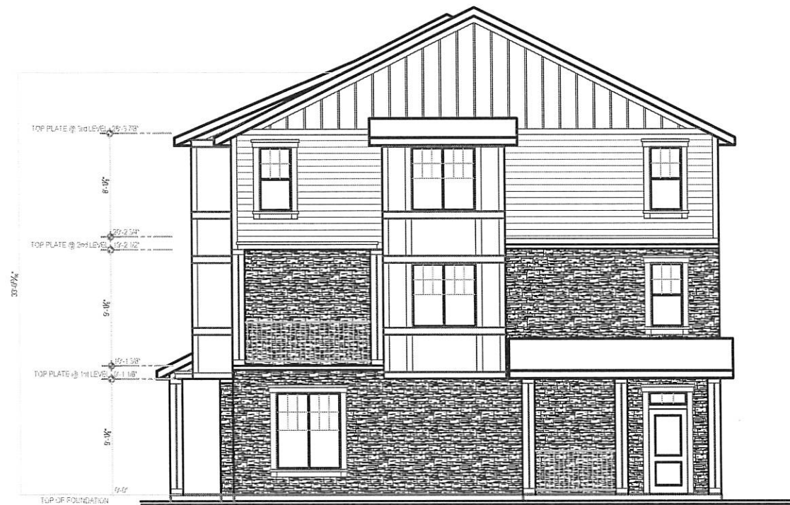
Front Buildings - Side Elevation
