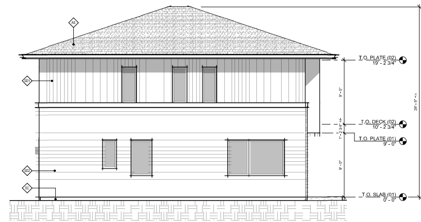
SOUTH (SIDE) ELEVATION (A3) 1/4" = 1'-0" AE201C
