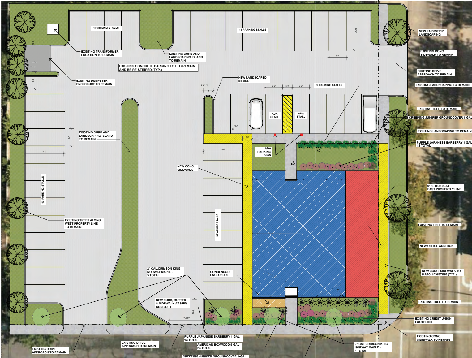
390 S. Main - Office Addition/Remodel - SITE PLAN Scale: 1" = 10'-0"
