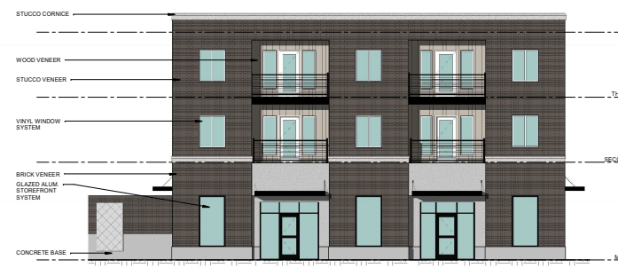
01 SW BUILDING - WEST ELEVATION 1/8" = 1'-0"
