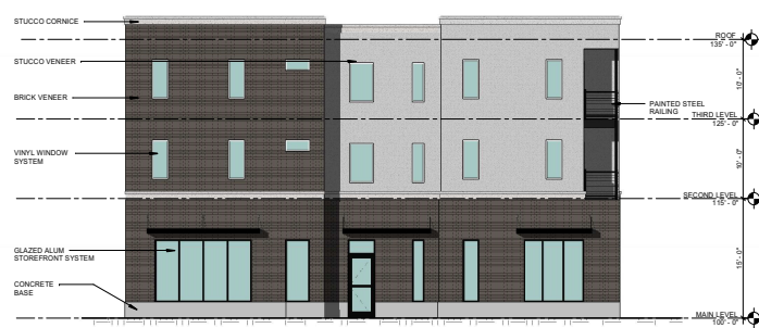
02 SW BUILDING - SOUTH ELEVATION 1/8" = 1'-0"
