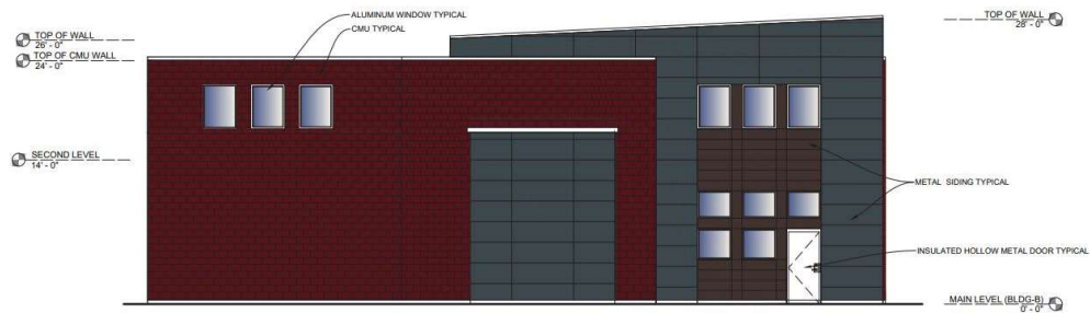
1 WEST ELEVATION 1/8"=1'-0" FULL SCALE 1/4"=1'-0" TYPICAL SCALE 1/8"=1'-0"
