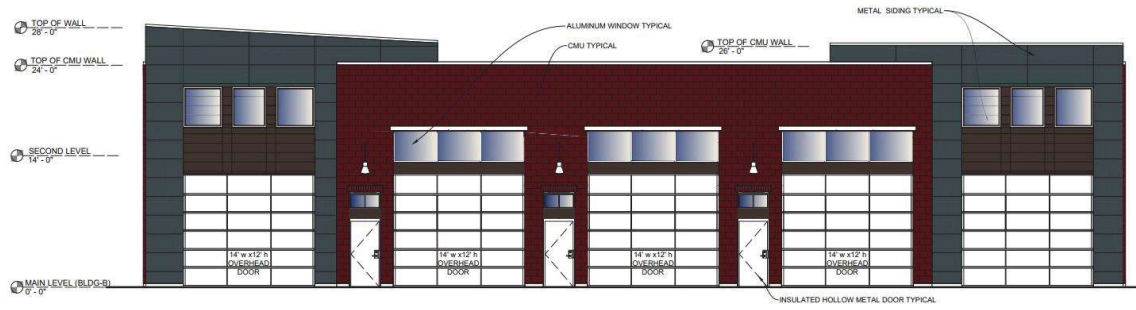
1 SOUTH ELEVATION 1/8"=1'-0" FULL SCALE 1/4"=1'-0" TYPICAL SCALE 1/8"=1'-0"
