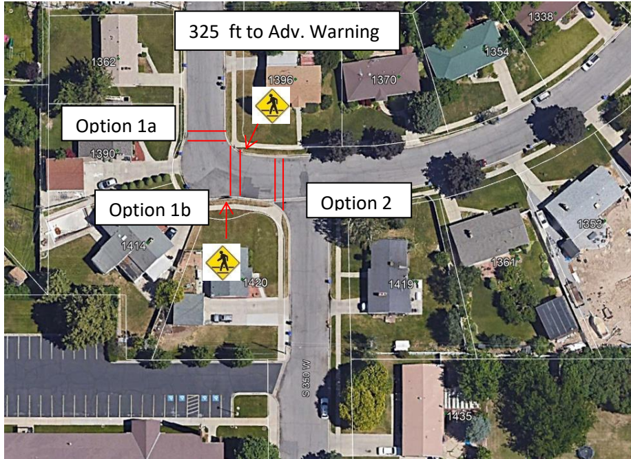
Figure 1 350 W / 1400 S intersection with proposed crosswalk configuration.
