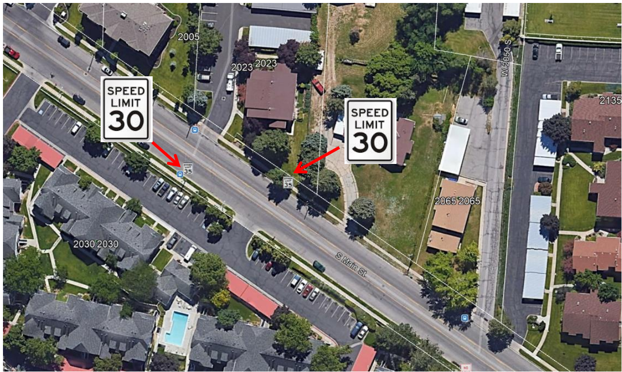
Figure 3 Replace existing 35 mph signs with 30 mph signs
