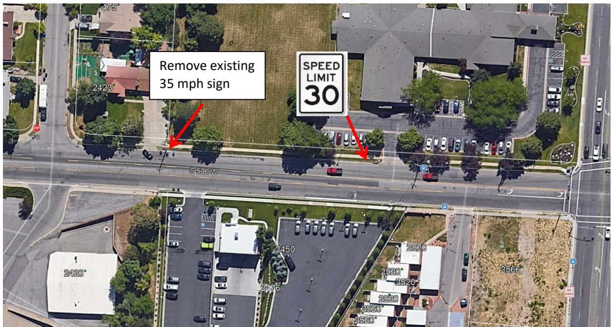
Figure 4 Remove existing 35 mph sign and install new 30 mph sign
