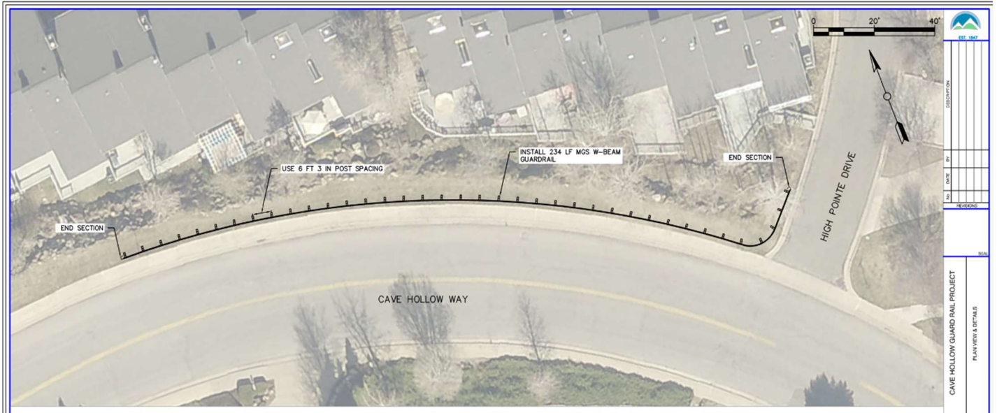
Figure 1 Proposed Guard Rail Installation
