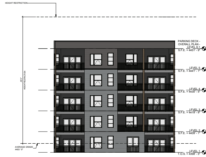
1 BUILDING 3000 COURTYARD ELEVATION - WEST 1/8" = 1'-0"
