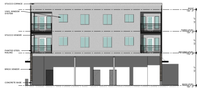
03 SW BUILDING - EAST ELEVATION 1/8" = 1'-0"
