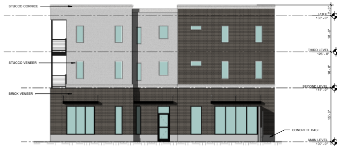
04 SW BUILDING - NORTH ELEVATION 1/8" = 1'-0"
