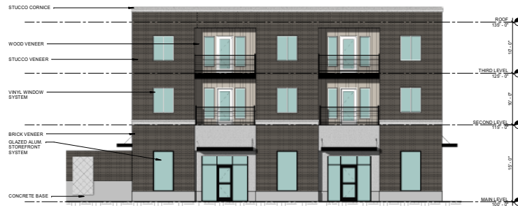
01 SW BUILDING - WEST ELEVATION 1/8" = 1'-0"
