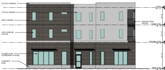
02 SW BUILDING - SOUTH ELEVATION 1/8" = 1'-0"
