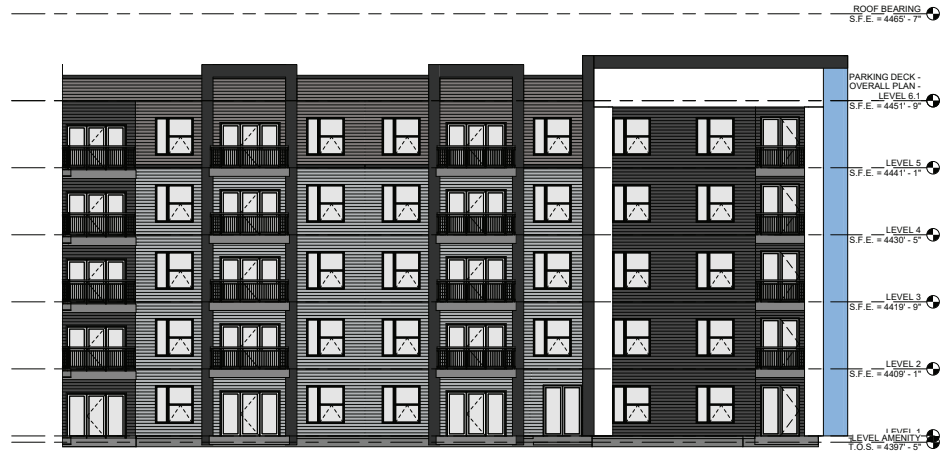
3 BUILDING 2000 COURTYARD ELEVATION - NORTH 1/8" = 1'-0"
