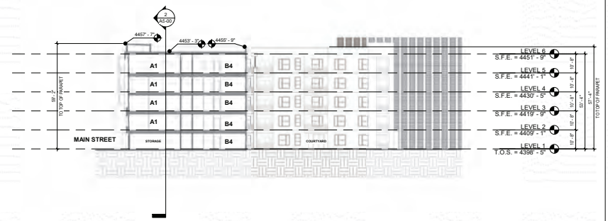
1 OVERALL BUILDING CROSS SECTION BLDG 1000 1" = 20'-0"
