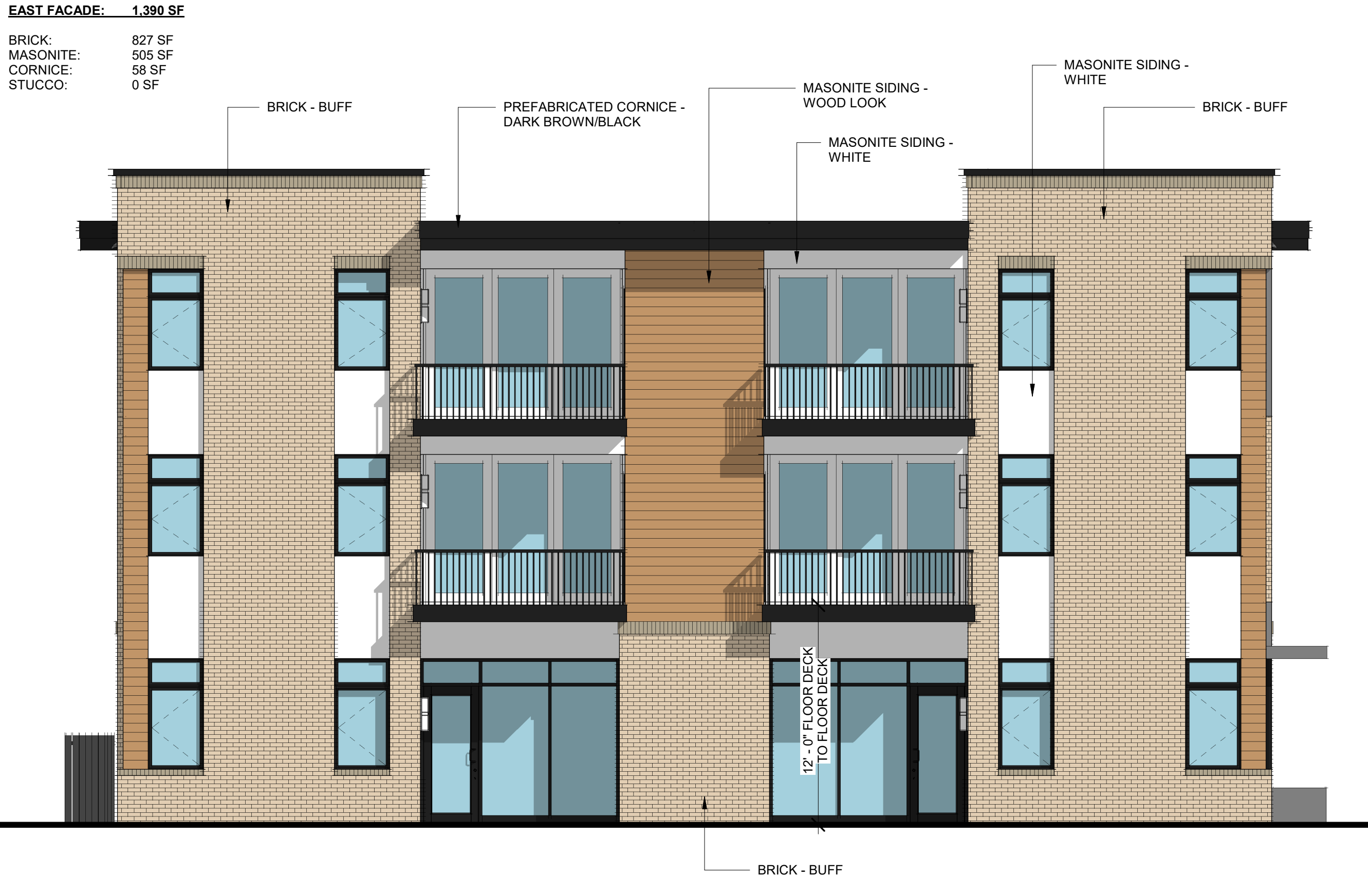
EAST (MIDDLE & WEST DRIVEWAY) ELEVATIONS A5 3/16" = 1'-0" AS109
