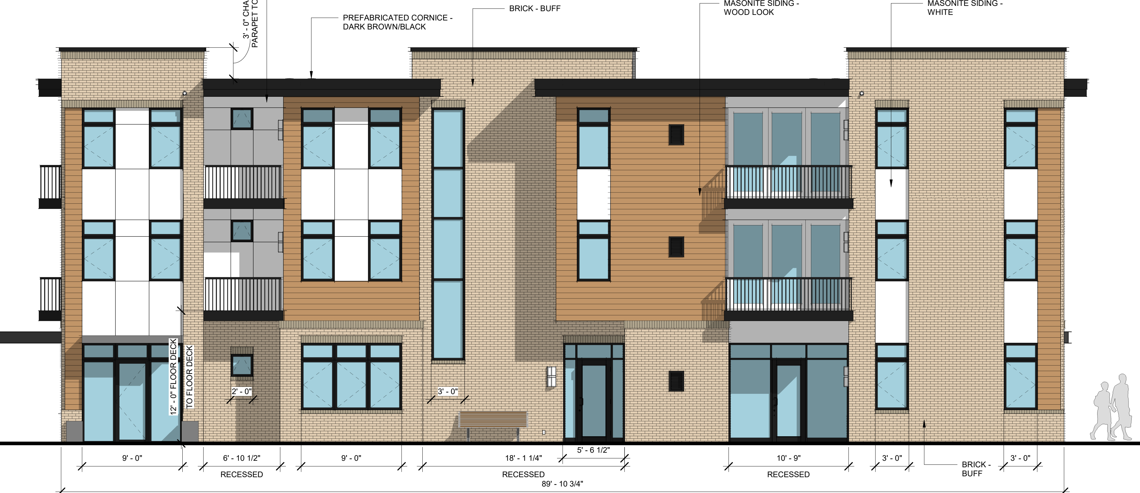
NORTH (400 SOUTH) ELEVATION A5 3/16" = 1'-0" AS108
