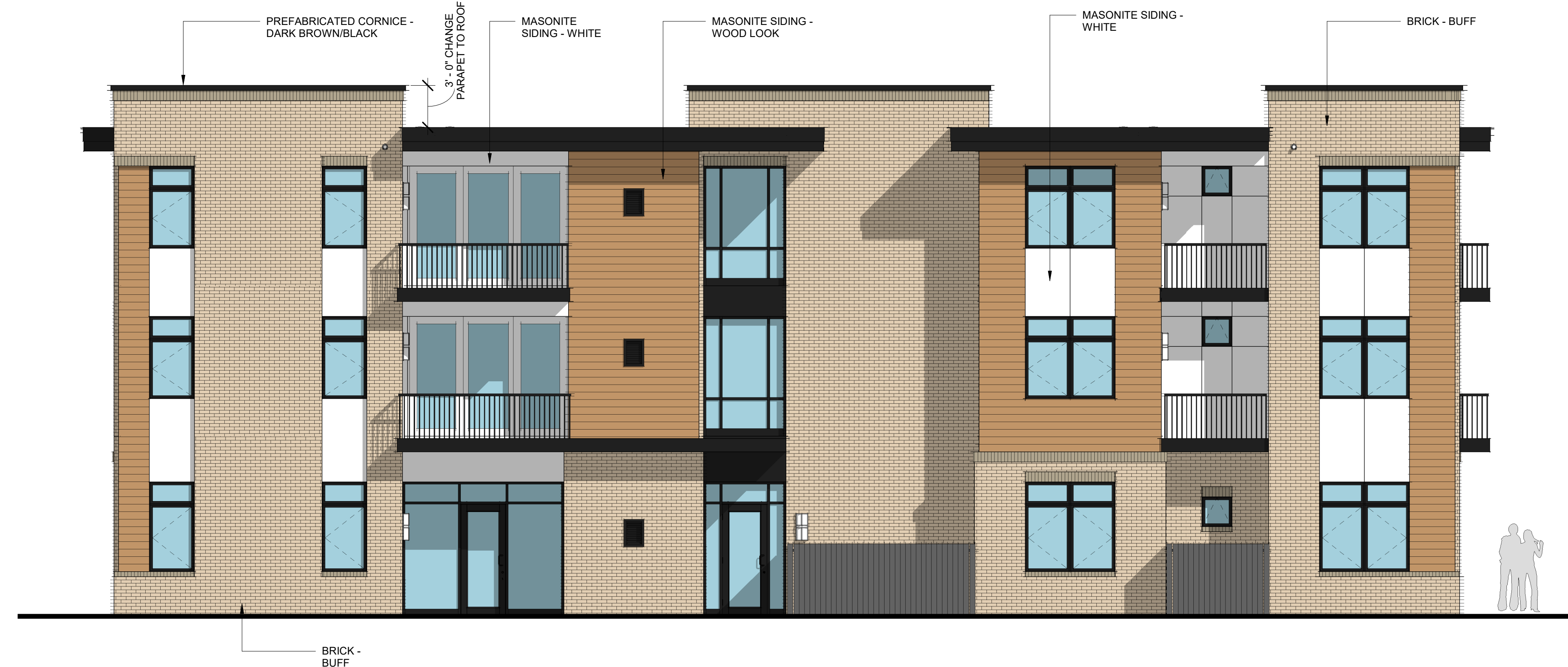
SOUTH (PARKING) ELEVATION C5 3/16" = 1'-0" AS108
