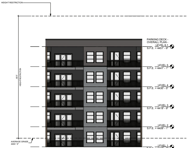
4 BUILDING 3000 COURTYARD ELEVATION - NORTH 1/8" = 1'-0"
