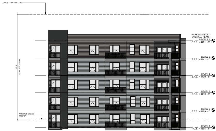
3 BUILDING 1000 COURTYARD ELEVATION - SOUTH 1/8" = 1'-0"
