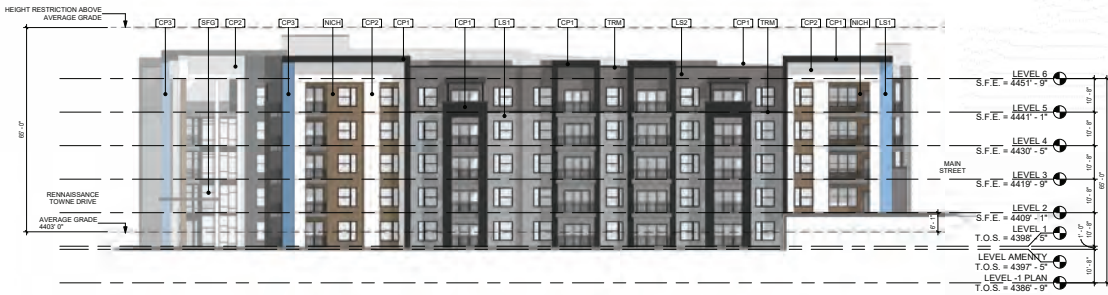
3 OVERALL BLDG. ELEVATION - SOUTH 1/16" = 1'-0"
