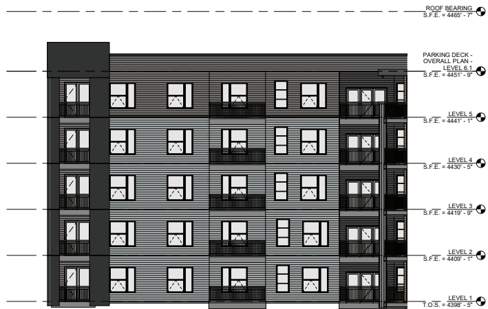
3 BUILDING 1000 COURTYARD ELEVATION - SOUTH 1/8" = 1'-0"
