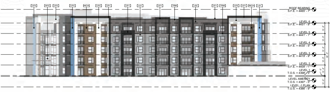
3 OVERALL BLDG. ELEVATION - SOUTH 1/16" = 1'-0"
