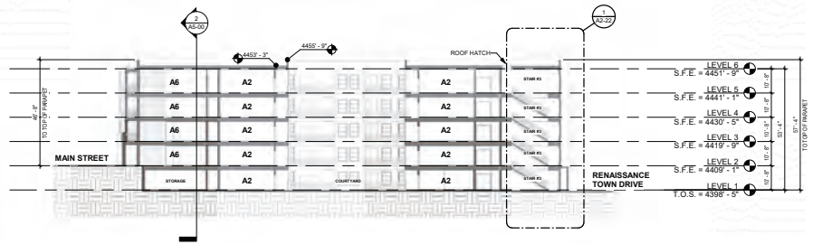
3 OVERALL BUILDING CROSS SECTION BLDG 3000 1" = 20'-0"
