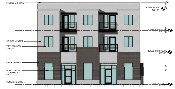
01 NW BUILDING - WEST ELEVATION 1/8" = 1'-0"
