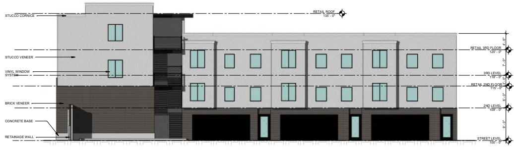
03 NW BUILDING - SOUTH ELEVATION 1/8" = 1'-0"
